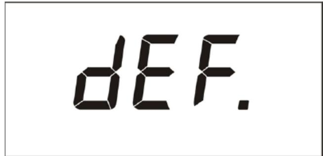
At this point, in order to perform a **partial RESET** (saving the calibration of the instrument), press the following keys in the order indicated:
