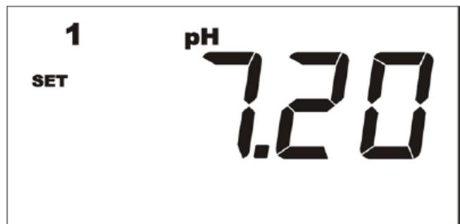
Defining the type of actuation is the next step: the down arrow indicates that the action tends to lower the measurement value (in the case of pH it represents an actuation of the acid type), the up arrow indicates that the actuation tends to increase the measurement value (in the case of pH it represents an actuation of the alkaline type).
