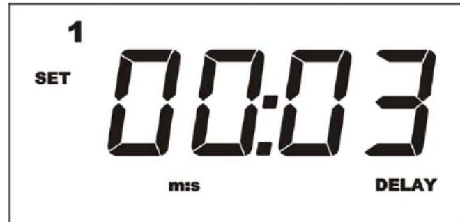
select the field to change (minutes or seconds) and confirm the choice by pressing the
