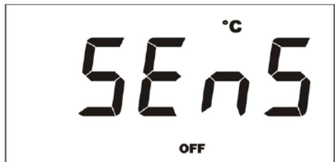
If the manual function (SenS off) is selected, the instrument's display shows the default
