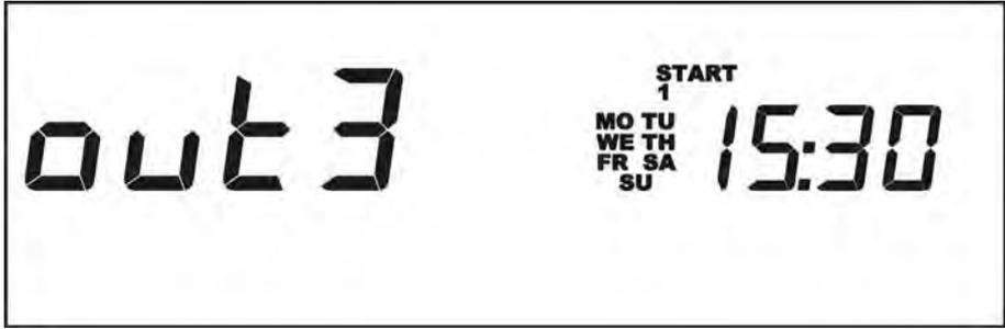
Once one of the two functions is activated (flocculant or cleaning) it is necessary to set the auxiliary outputs that need to be activated.
