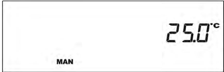
temperature value can be set in the range between 0 and 99.9°C. Press the
