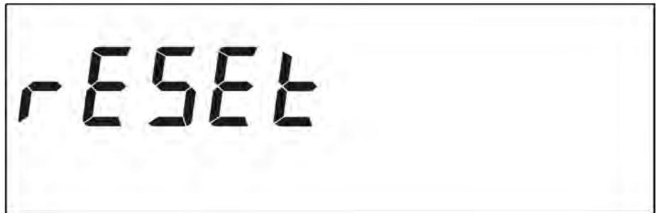
At this point, in order to perform a **partial RESET** (saving the calibration of the instrument), press the following keys in the order indicated:
