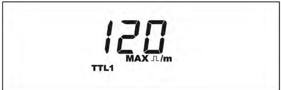
As soon as the maximum frequency value is set, the minimum frequency value, corresponding to SETPOINT actuation must be set.
